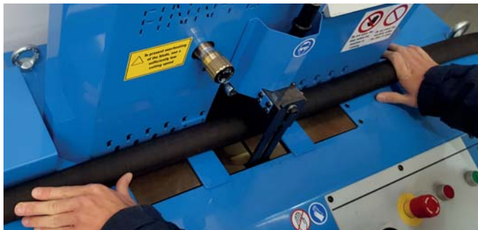
Figure 10: A photograph showing how to cut hydraulic hose using a dedicated hose cutter.
