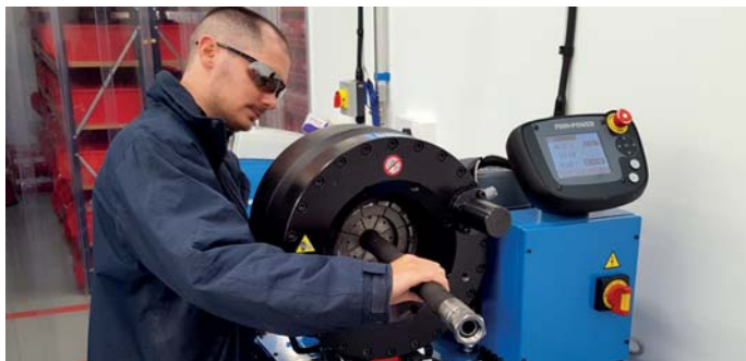
Figure 12: A technician swaging a hydraulic hose assembly using a swaging machine.
