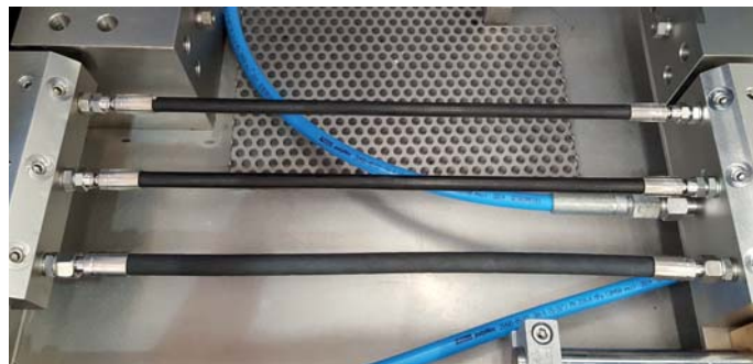
Figure 13: A photograph showing 3 hoses attached to a hydrostatic test bench before testing.
